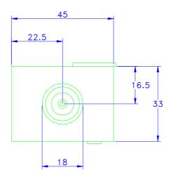
Material: Body, Carp grade Tufnol Mounting Boss: 18mm Diameter Connector: TNC Socket (Female) Tolerance: ±0.1mm
